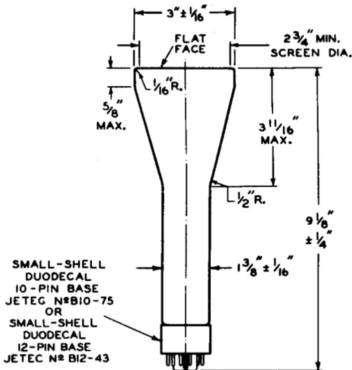
CENTER LINE OF BULB WILL NOT DEVIATE MORE THAN 2° IN ANY DIRECTION FROM PERPENDICULAR ERECTED AT CENTER OF BOTTOM OF BASE.
